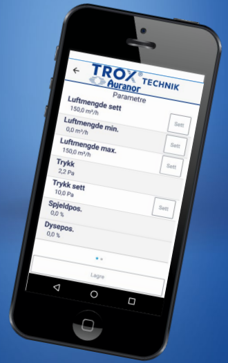
The app TROX ECA can be used for commissioning and service. The app communicates wireless with phone or tablet by Bluetooth.
