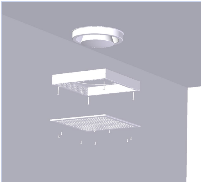
Fig.5, installation of Gitter-F
