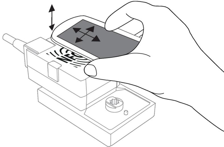
**Tool connection** The actuator can be parametrised by ZTH EU via the service socket. For an extended parametrisation the PC tool can be connected.
