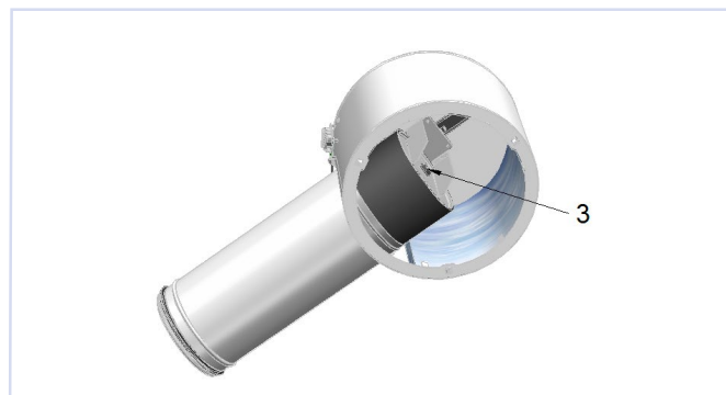
Figure 9, Remove the wing screw (6 mm) from the damper (3) and pull the damper bracket into the rear position. The actuator and damper are now loose from the casing.(MI)
