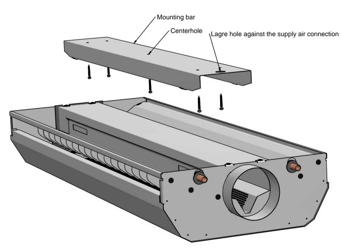
The mounting bar is fitted on Svalbard-F.
